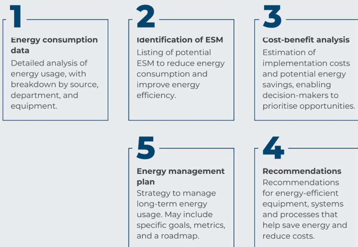
Typical structure of an energy audit report.
